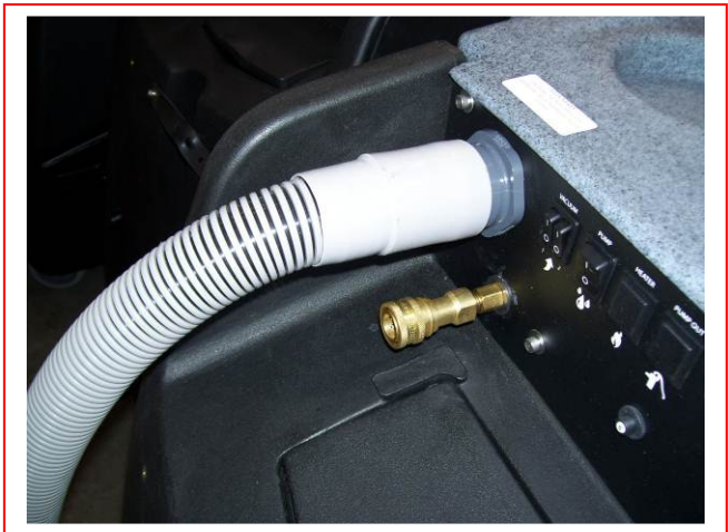
Vacuum Hose Connection with standard barb and vinyl cuff
