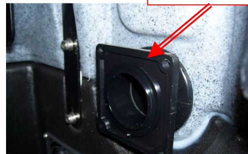
Unless damaged or leaking between tank and flange, the flange fitting does not have to be removed
