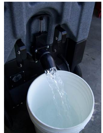
Draining the Recovery Tank
